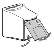
5 Connect the power cord to the wall outlet after you complete all the connections.
